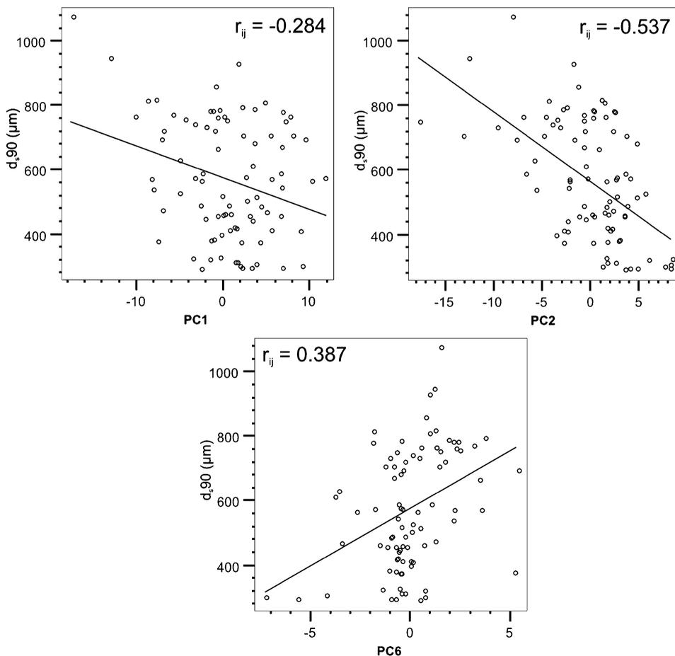
Figure 3. Scatter plots showing the Pearson correlation coefficients ( $r_{ij}$ ) of Table 2 between  $d_{s,90}$  and the principal components (PCs). Correlation coefficients and scatter plots between  $d_{s,10}$ ,  $d_{s,50}$  and PC2 and PC6 are very similar; as such scatter plots are not presented. Correlation coefficients between the silt-clay% and PC2 and PC6 are very weak. As such, those scatter plots are not presented.
