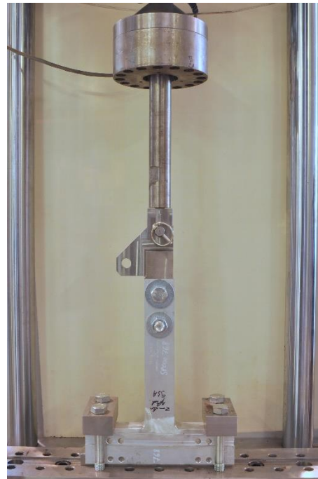
Figure 2: Fatigue testing of welded aluminum T-joint
