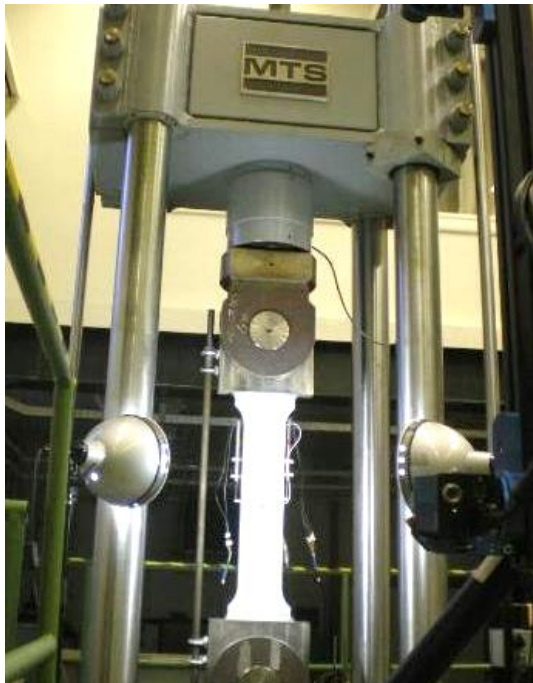
Figure 1: Medium wide plate tension test in MTS 2500
